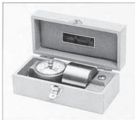
for hardness tests in compliance with the standards according to Shore A, B, O, OO and Shore D, C, DO.
